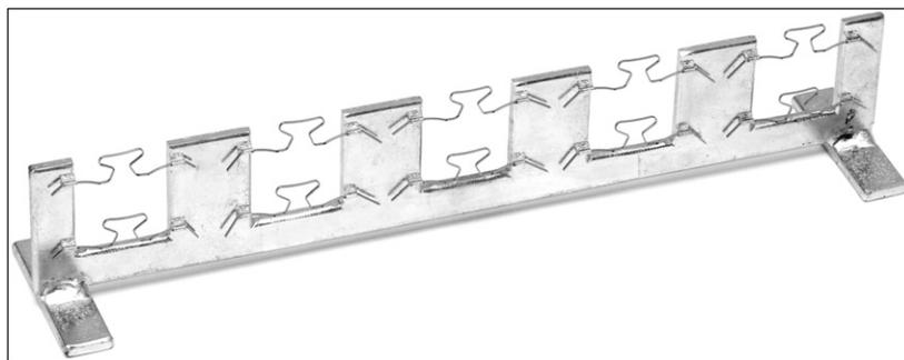
**Fig 4.** Custom-made device to keep the TLSs activated at 5 mm.
