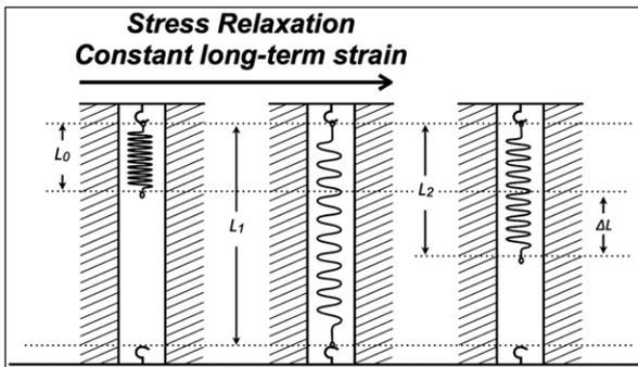
**Fig 1.** Stress relaxation test in a helical spring.  $L_0$ , Original length;  $L_1$ , extended length due to activation (constant strain);  $L_2$ , total length after stress relaxation;  $\Delta L$ , deformation due to stress relaxation.
