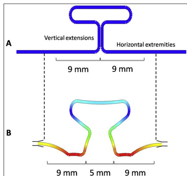
**Fig 5.** **A**, Loop regions and dimensions on the horizontal extremities used to ensure the correct activation and the centralization of the TLS; **B**, TLS shape when positioned symmetrically in an interbracket distance of 23 mm and activated 5 mm.
