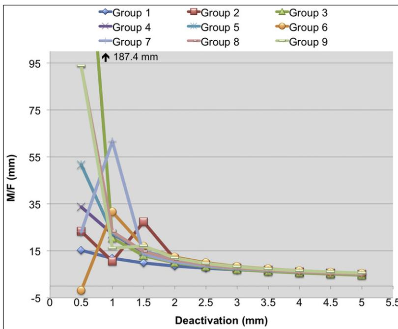
**Fig 8.** Chart depicting the average MF ratios produced during deactivation from 5 to 0.5 mm for the groups tested.
