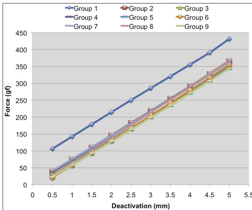
**Fig 6.** Chart depicting the average forces produced during deactivations from 5 to 0.5 mm for the groups tested.
